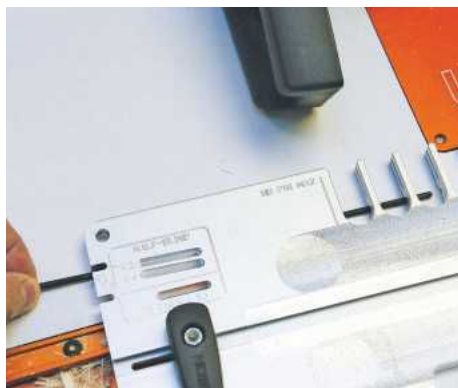
▲ This black rod slides into a channel on the jig
